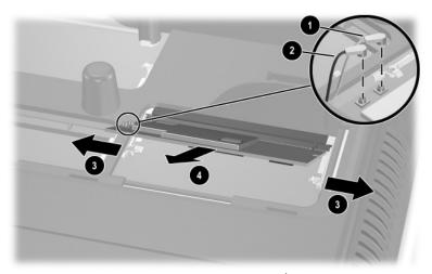
Removing a Mini PCI Communications Board
